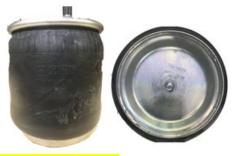
Note: Plastic Piston and Steel Piston ZMD air springs can be mixed.
