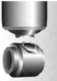
Damaged upper or lower mount
