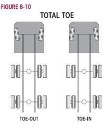
**Toe-out on Turns** — (See Ackermann Geometry). Excessive turning angles such as those encountered in pickup and delivery operations may contribute to premature tire wear. Be advised that the greater turning angles, the more that toe and camber change. If you have any doubt regarding the optimum turning angles for your operation, contact the vehicle's manufacturer, axle OEM, tire OEM and alignment equipment manufacturer for advice.
