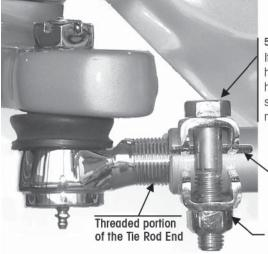
5/8" Tie Rod Clamp Bolt It is critical to check the 5/8" tie rod clamp bolt head location to verify the clamp fasteners have sufficient clearance away from the lower shock mount at full wheel cut. The fasteners must not contact the lower shock mount.
