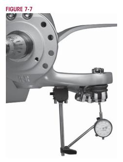
According to the Commercial Vehicle Safety Alliance (CVSA), the "out of service" criteria for front steer axle tie rod assemblies on any commercial vehicle is: Any motion other than rotational between any linkage member and its attachment point of more than ½" (3 mm) measured with hand pressure only. (393.209(d)), (published in the North American Standard Out-of-Service Criteria Handbook, April 1, 2006.)
