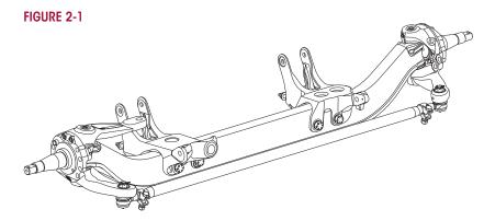
Hendrickson's next generation lightweight, fabricated STEERTEK NXT axle for the International Truck MaxxPower Front Air Suspension combines rigid strength with outstanding maneuverability. Chosen by many OEMs as the standard axle for select vehicle models, STEERTEK NXT is approved for use in on-highway and medium-duty truck, bus and motorhome applications. STEERTEK NXT's unique design provides up to 23 pounds of weight savings compared to traditional forged I-beam axles.
