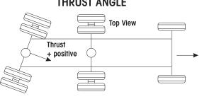
Thrust Angle, Tracking, or Square — The angle formed by the centerline of the vehicle frame (geometric centerline) and the direction that an axle points. As indicated by the term "square", the ideal value for the angle is 0° or when the axle centerline is at 90° or perpendicular to the geometric centerline. Thrust or tracking to the right is positive, and to the left is negative.
