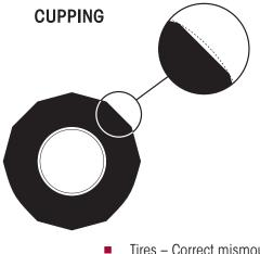
**Cupping** — Localized, dished out areas of fast wear creating a scalloped appearance around the tire. Cupping, which appears around the tire on the shoulder ribs, may also progress to adjoining ribs, see TMC RP 219A publication, page 7.
