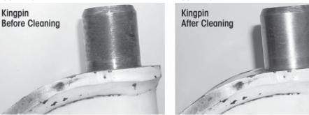
2. Inspect the kingpin for wear or damage. Use a micrometer and measure the upper and lower kingpin in two locations. Positions must be 90° opposed from each other. If the kingpin has less than 1.802" diameter, replacement of the axle is necessary, see Figures 9-7 through 9-10.
