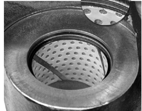
Magnification of King Pin Bushing and Lip seal installed in steering knuckle.
