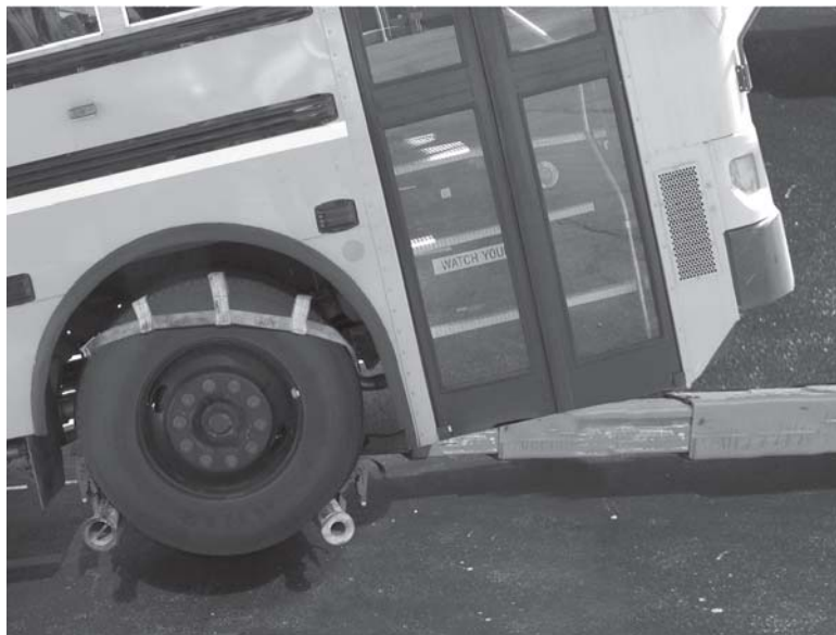
FIGURE 6-1 Wheel Lift Method
