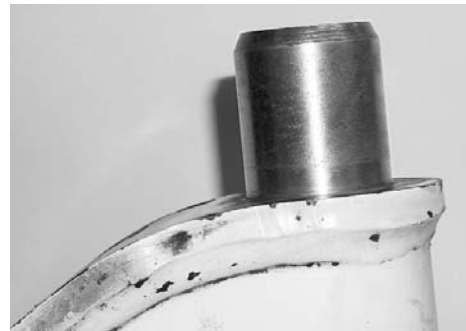
FIGURE 9-33 KINGPIN AFTER CLEANING
