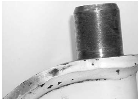
FIGURE 9-32 KINGPIN BEFORE CLEANING
