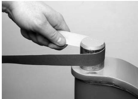
FIGURE 9-32 KINGPIN BEFORE CLEANING
