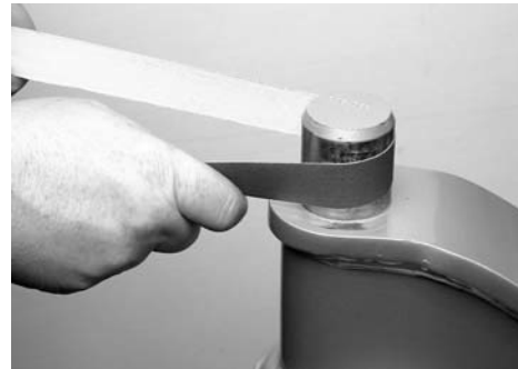
FIGURE 9-33 KINGPIN AFTER CLEANING
