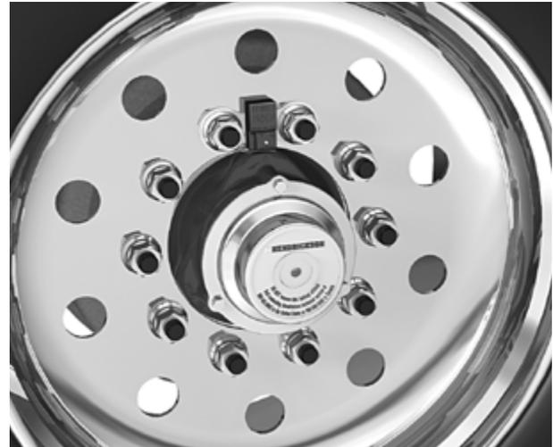
Figure 7: Properly installed WEM
