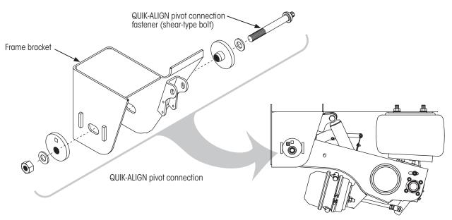
The current bolt features a round head that helps to prevent reuse. Applying the proper torque and clamp force at the pivot connection is the same as it has always been. Simply install the bolt from the inboard side of the frame bracket and tighten with a Torx<sup>®</sup> socket until the bolt's Torx head shears off. To avoid damaging the splines on the shear bolt's Torx head, make sure the drive socket fully engages the Torx head.
