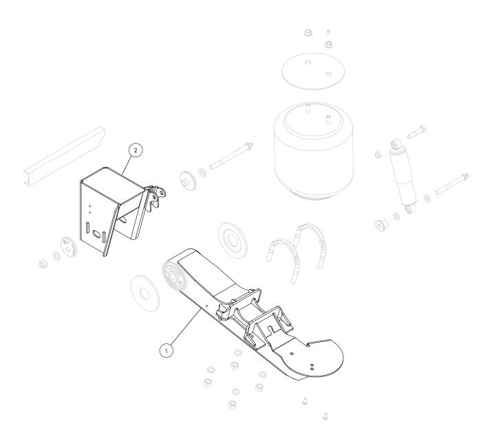
Wingless, weld-on frame bracket with QUIK-ALIGN® (Shown)
