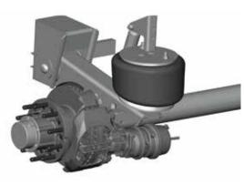
B. For top-mount air suspensions with brake chamber to the FRONT of the axle.
