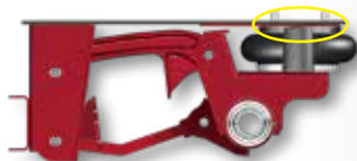
Figure A: Primary (airbag) bump stop engages
