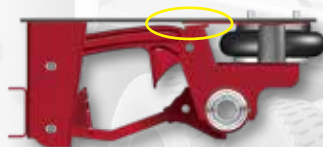
Figure B: Under extreme load, secondary bump stop engages
