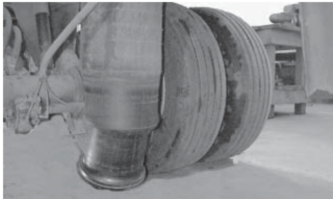
Figure 6. Check clearance underneath the trailer
