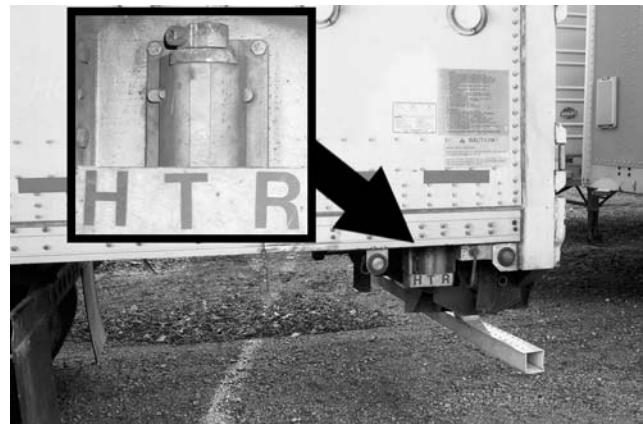
Figure 3. Trailer mode valve
