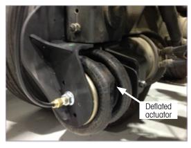
**Step 3:** Remove outboard lift actuator mounting plate bolt and nut.
