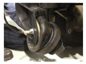
Step 6: Insert caging tool as shown. Tool may need to be inserted at an angle in order to fit into slot.
