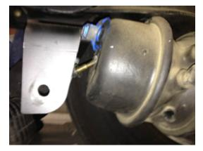
Step 8: Tighten caging tool until spring is compressed and brakes are released.
