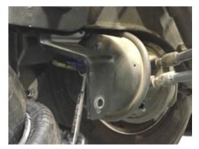
End of procedure: Brake chamber shown fully caged.
