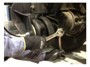
**Step 1:** Suspension lowered and air exhausted from lift actuators.
