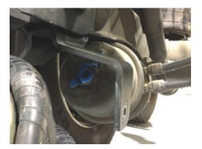
Step 7: Using 34" wrench, run caging tool nut snug against chamber housing. Continue turning to compress spring.
