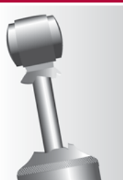
Damaged dust cover and / or shock body
