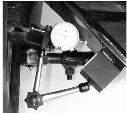
7. **CHECKING THE LOWER KINGPIN BUSHING.** Install a dial indicator so that the base is on the axle and the indicator tip is against the inside of the bottom of the knuckle. See Figure 7-21.
