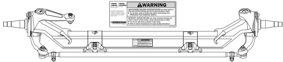
THE STEERTEK HAS A UNIQUE AXLE. THE KINGPIN IS CRYOGENICALLY INSTALLED IN THE AXLE. THE KINGPIN IS A NON-REPLACEABLE COMPONENT OF THE AXLE ASSEMBLY. DO NOT TRY TO REMOVE THE KINGPIN. IF THE KINGPIN SHOWS SIGNS OF MOVEMENT, CONTACT THE HENDRICKSON TECH SERVICE DEPARTMENT.
