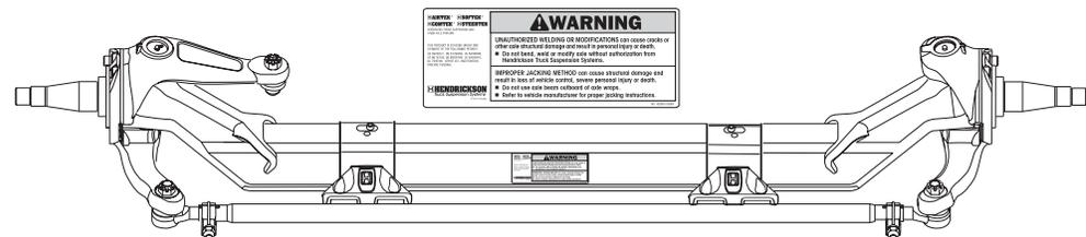
7. Check and adjust caster angle. Refer to "Caster" in the Definitions under the Alignment & Adjustments Section of this publication. **The use of two different angle caster shims will not change cross caster.** Cross caster is the difference between the caster readings for left and right side of the vehicle.
