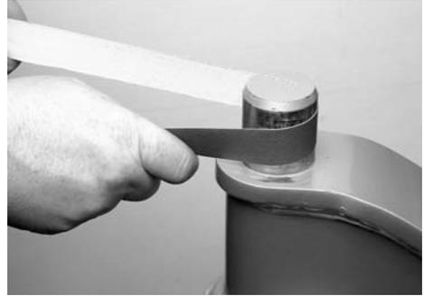
**FIGURE 9-35 KINGPIN BEFORE CLEANING**
