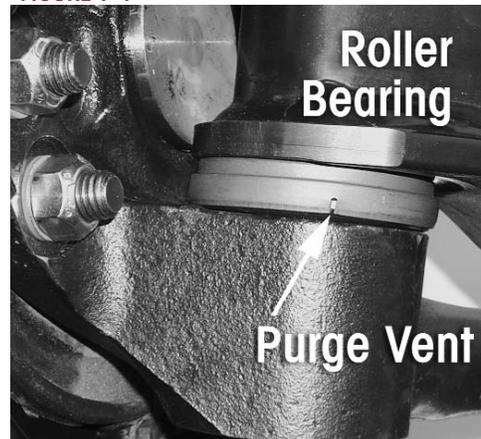
**NOTE** Greasing at the lower zerk should purge grease from the thrust bearing shell.
