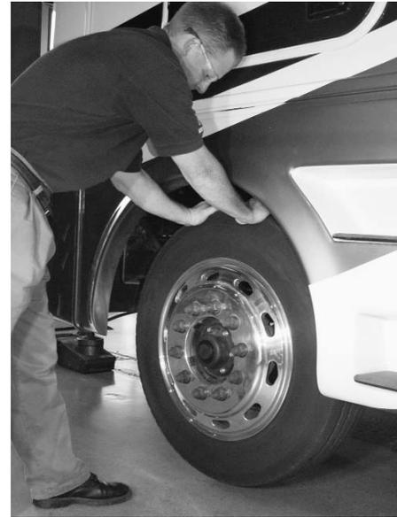
**STEERING KNUCKLE INSPECTION****CHECKING VERTICAL END PLAY (UP AND DOWN MOVEMENT)**
