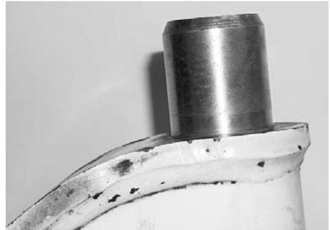
2. Inspect the kingpin for wear or damage. Use a micrometer and measure the upper and lower kingpin in two locations. Positions must be 90° opposed from each other. If the kingpin has less than 1.802" diameter, replacement of the axle is necessary, see Figures 9-37 through 9-40.
