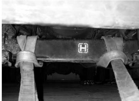
**FIGURE 3-3 NOT ACCEPTABLE**
