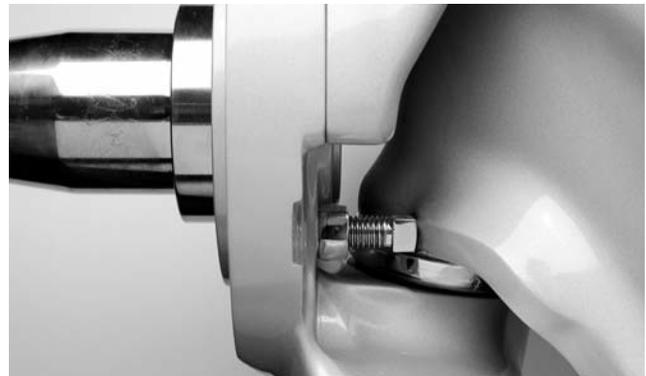
5. Decrease the wheel cut by loosening the jam nuts and screw the axle stops out counter-clockwise.
