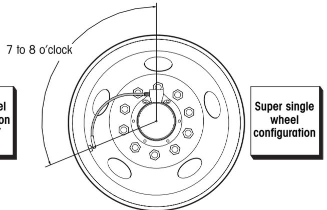
With the hubcap fitting in the 12 o'clock position, the valve stem should be located between 7 and 8 o'clock for most applications. When the wheel is installed, verify that the tire hose is not stretched so tightly that a strain is introduced at either the valve stem or hubcap fitting. Also make sure the tire hose is not so loose that it contacts the wheel.
