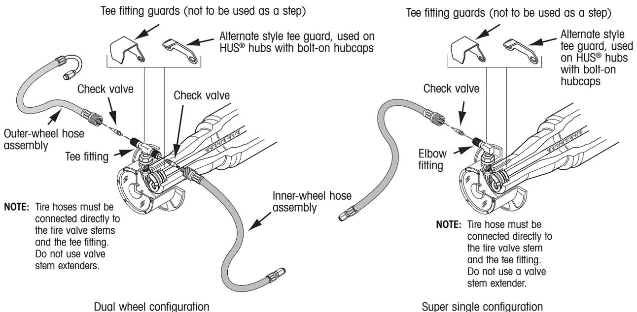
Figure 31. Tire hose, check valve and tee fitting guard installation
