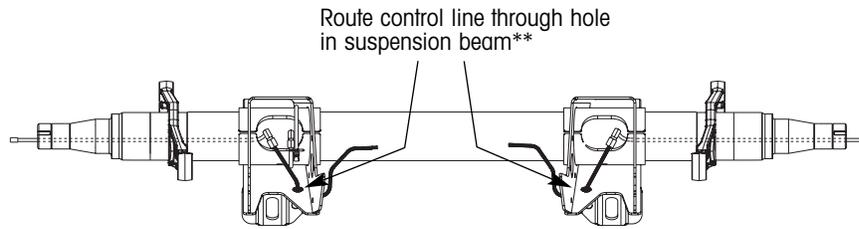
Figure 24. Suggested control line installation details for Low Ride, Wide Bushing, Standard Duty (AAL 23K, AAL 25K, AAZL, AAL 30K); Low Ride, Wide Bushing, Extreme Duty (AAEDL 30K); and Top Mount, Wide Bushing, Extreme Duty (AAEDT 30K) Models
