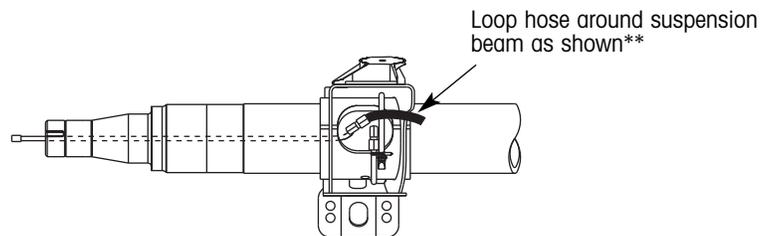
Figure 23. Suggested control line installation details for Top Mount, Narrow Bushing, Standard Duty Models (HKANT, AANT, AAZNT)
