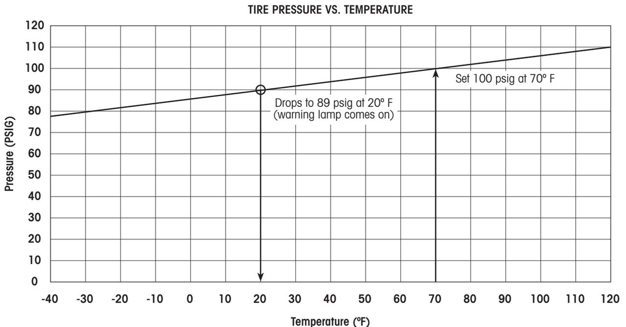
figure 41. Typical tire maintenance system performance at 100 psig
