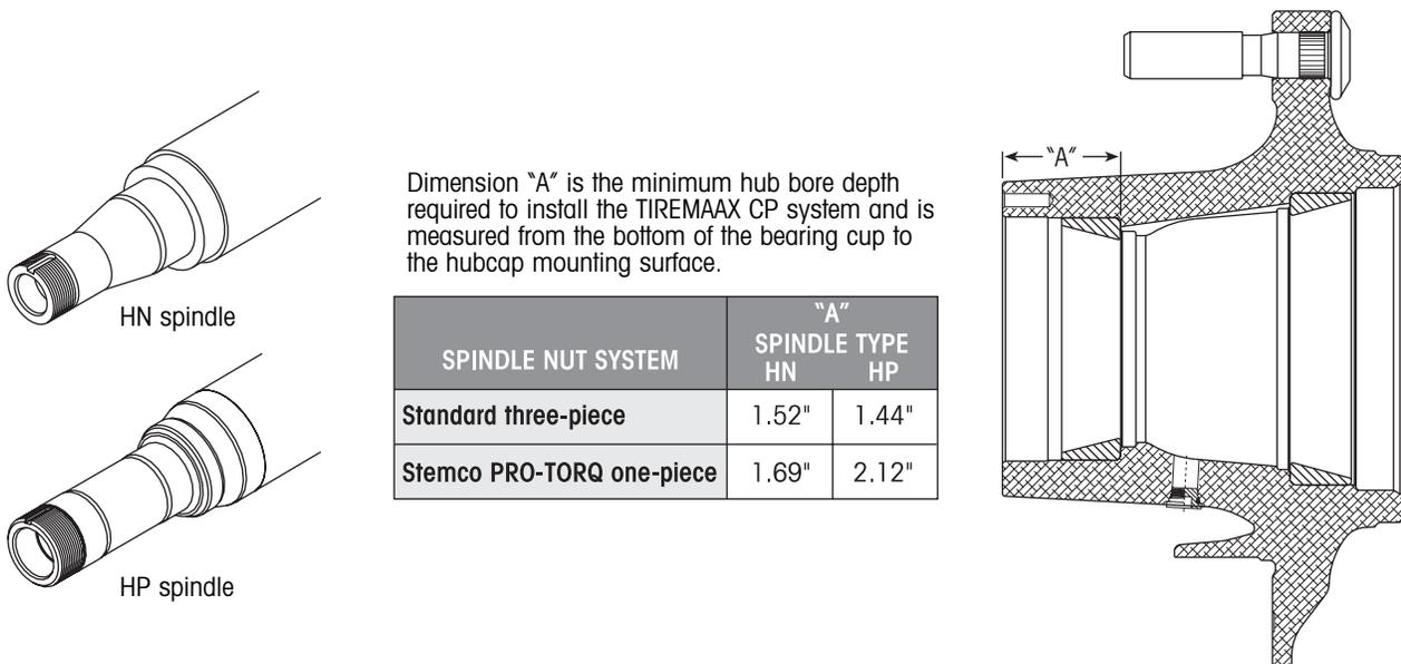
Figure 12. Minimum hub bore depth
