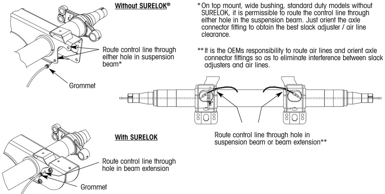
Figure 22. Suggested control line installation details for Top Mount, Wide Bushing, Standard Duty Models (AAT, HKAT)
