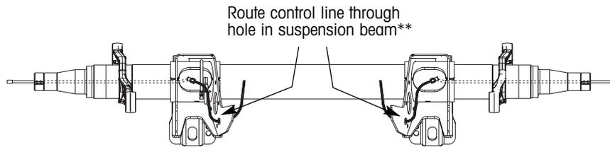
Figure 25. Suggested control line installation details for Low Ride, Short Beam, Narrow Bushing, Standard Duty Models (AANLS 20K)
