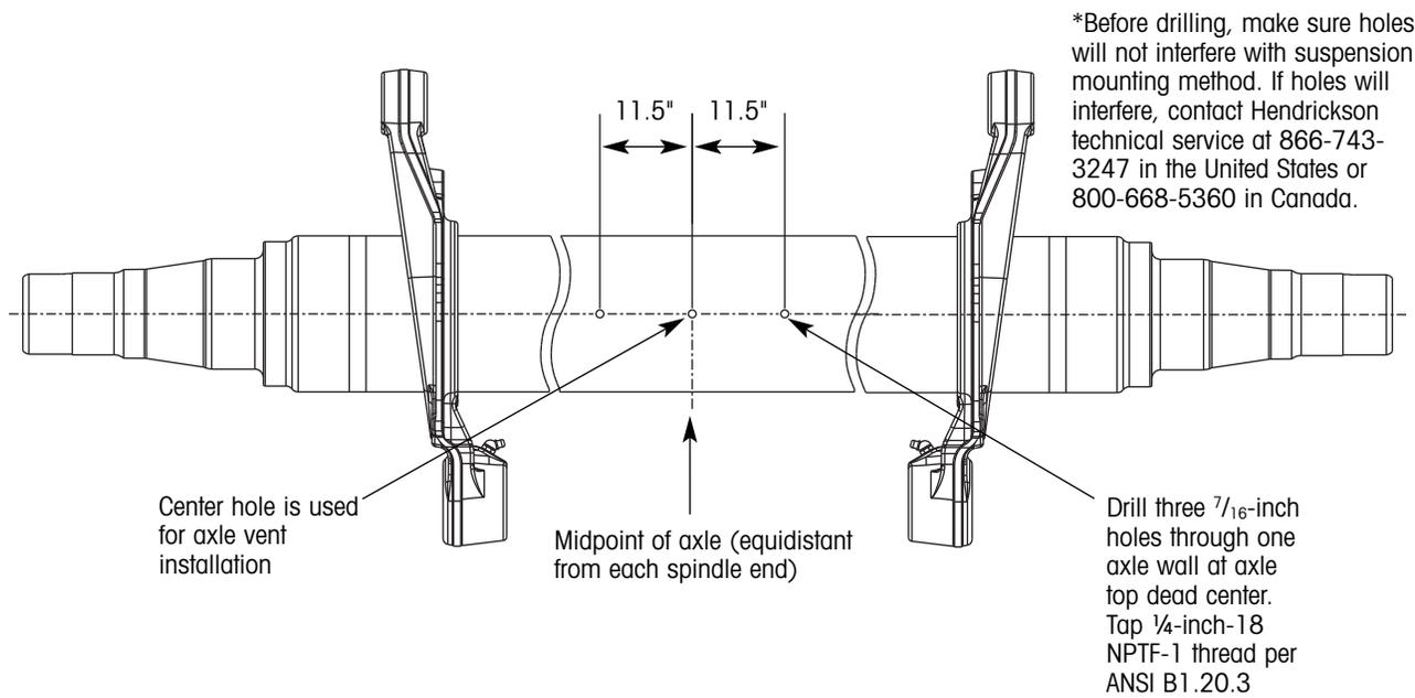
Figure 7. Hendrickson Trailer Axle drilling details
