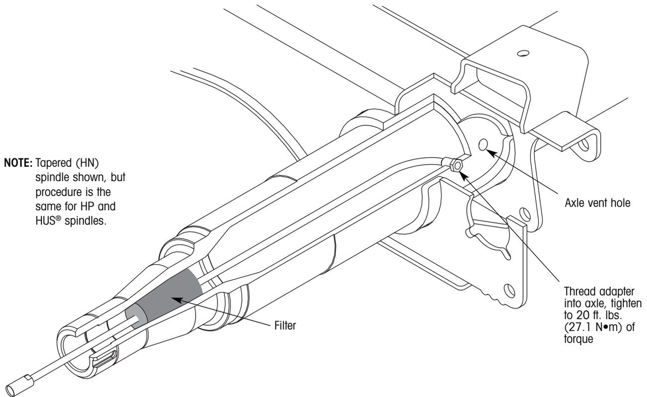
Figure 9. Installed position of hose assembly
