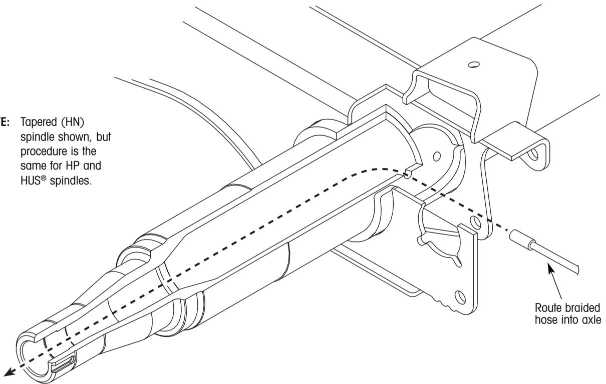
Figure 8. Routing hose in axle
