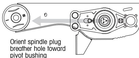
Orient spindle plug breather hole toward pivot bushing
