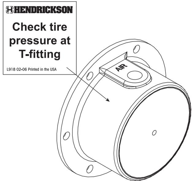
Figure 34. Recommended decal mounting location
