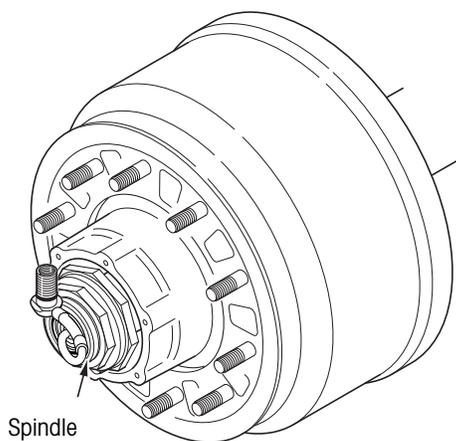
Figure 17. Completed installation of rotary joint assembly
