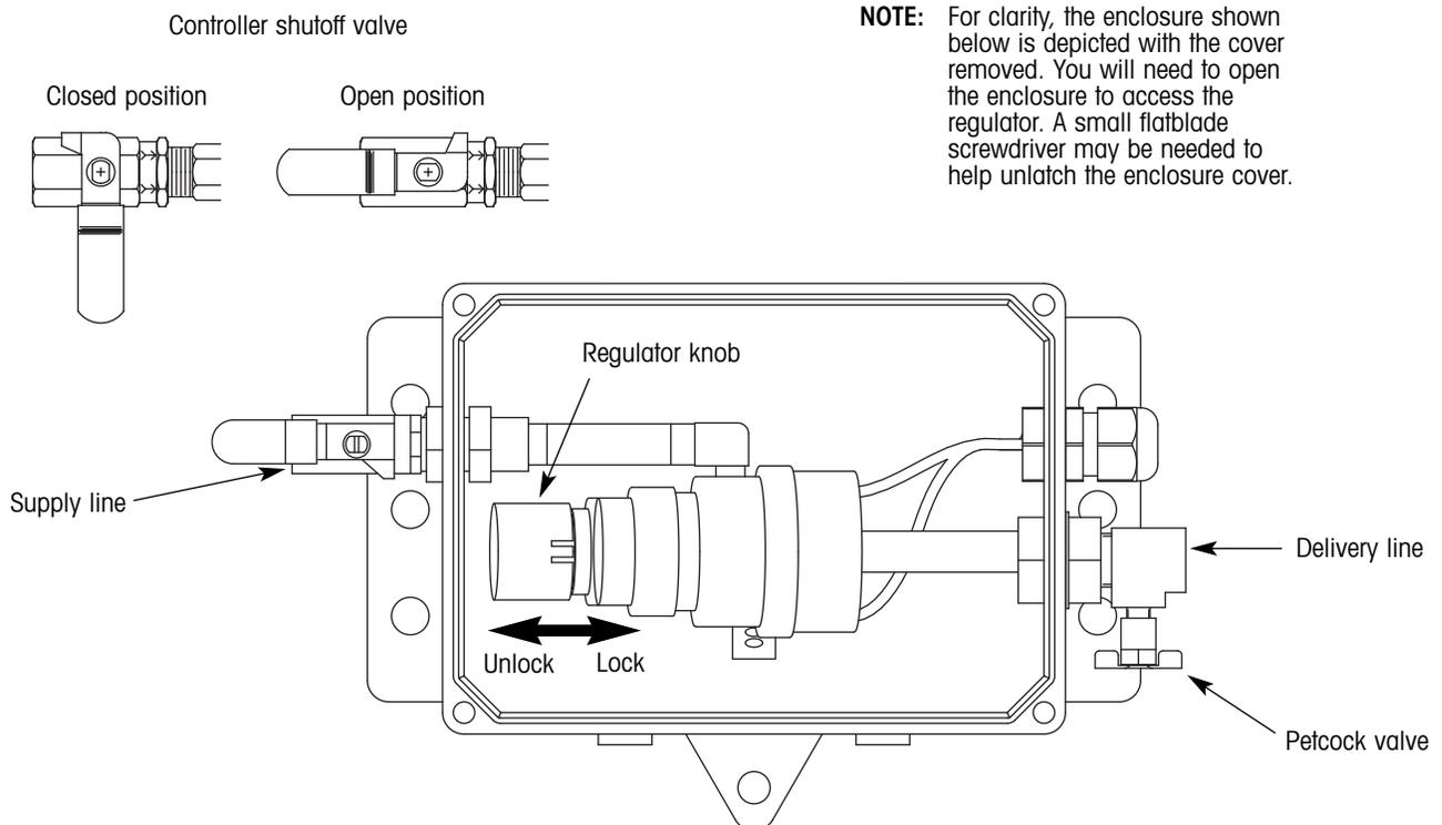
**NOTE:** For clarity, the enclosure shown below is depicted with the cover removed. You will need to open the enclosure to access the regulator. A small flatblade screwdriver may be needed to help unlatch the enclosure cover.
