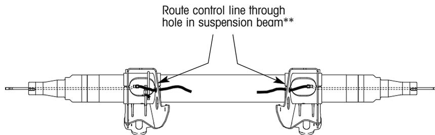
Figure 25a. Suggested control line installation details for Low Ride, Narrow Bushing, Standard Duty Models (AANL)
