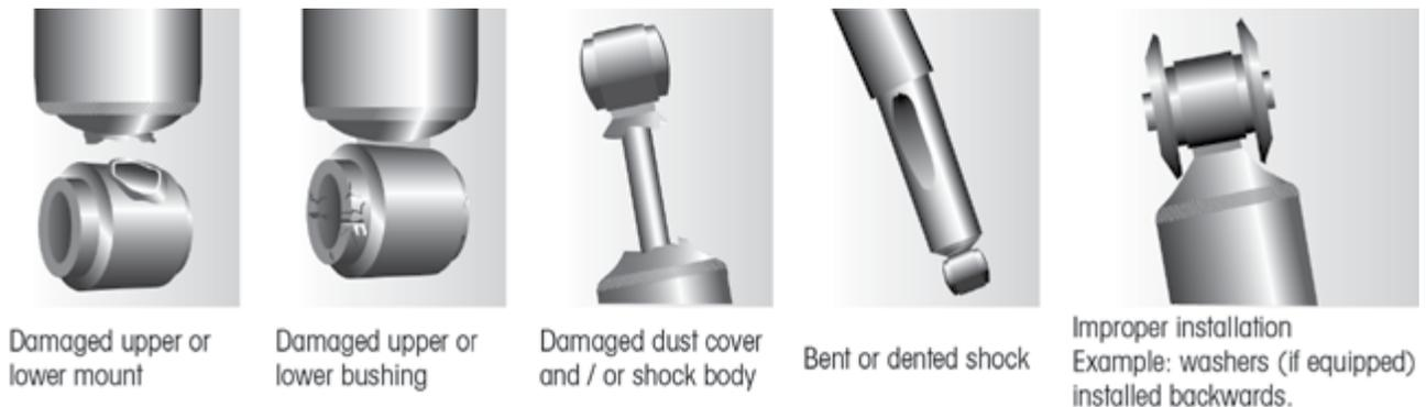
**LEAKING VS. MISTING SHOCK ABSORBER VISUAL INSPECTION**
