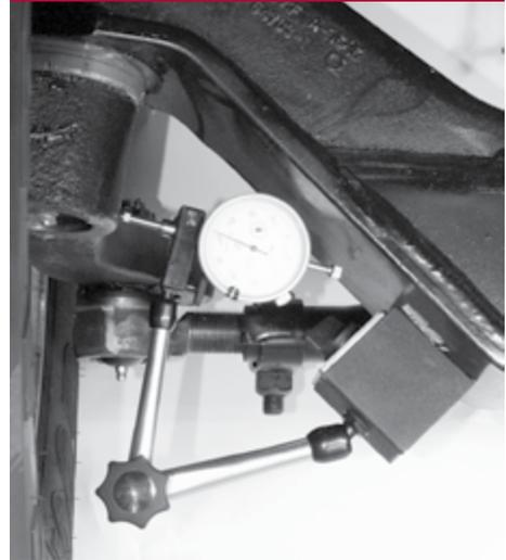
9. Move the bottom of the tire in and out. If the dial indicator moves more than 0.015", the lower bushing is worn or damaged. Replace both kingpin bushings. Refer to the Component Replacement Section of this publication.
