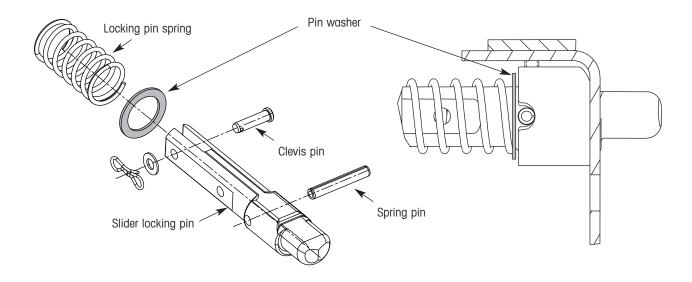
To install the pin washer, the clevis pin and spring pin must be removed. With these pins removed, the slider locking pin can be pushed outboard through the slider frame rail and removed, along with the locking pin spring. A suggested tool to help remove the spring pin is shown below. Dimensions have been included so it can be fabricated locally (it is not available for purchase).
