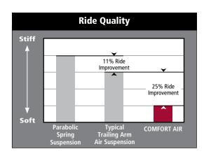
Using advanced spring technology from Hendrickson, COMFORT AIR's main support member has an elongated design for optimized roll stiffness. This provides a softer ride and greater protection from the effects of road shock on your chassis, equipment, drivers and passengers.
