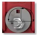
Maximum range of adjustment is ± 90 degrees from 12 o'clock positioning.
