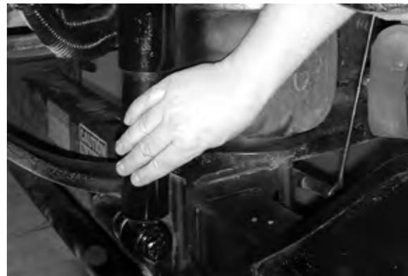
2. Use an infrared thermometer to check the temperature of the shock absorber. This can also be performed by carefully touching the shock absorber body below the dust cover. Touch the frame to get an ambient reference, see Figure 7-21. A warm shock absorber is acceptable, a cold shock absorber should be replaced.
