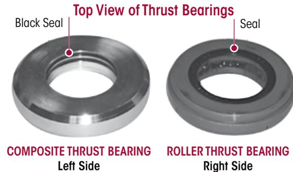
1. Install the thrust bearing on the lower kingpin with the seal facing up toward axle (the black seal will designate the top side, see Figure 9-45). The composite thrust bearing is installed on the left side of the axle. The roller bearing is installed on the right side of the axle.
