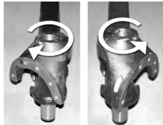
5. Clean and remove all kingpin bushing material from the steering knuckle assembly. Take special attention to remove material from the grease channels and dimples.
