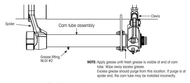
Figure 4: Cam tube weld mount assembly (top view)
