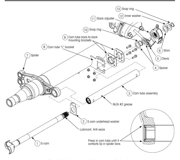
Figure 3: Cam tube system part identification and weld information
