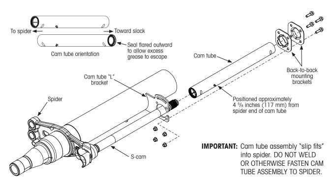
Figure 1: Cam tube assembly installation overview
