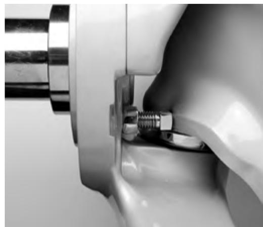
**NOTE** It is very important that the sides of the square head axle stops are set parallel to the axle beam to ensure a good contact point on the axle, see Figure 8-15.
