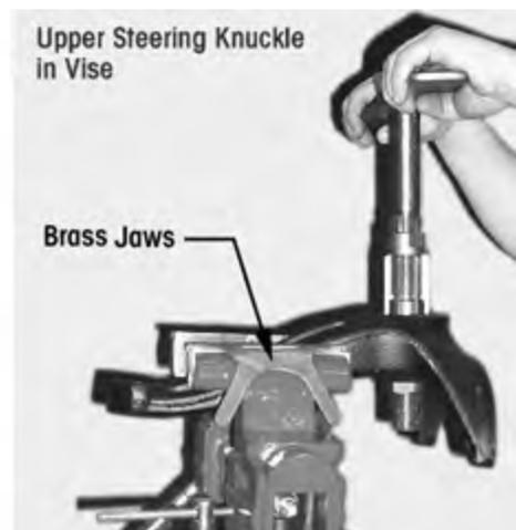
7. Install the steering arm and upper kingpin connection on the kingpin.
