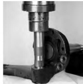
3. Use the Kingpin Handle and Bushing Driver Installer / Remover Tool to sink the kingpin bushing to just below the seal bore, see Figures 9-30 to 9-32.
