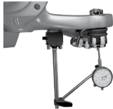
10. Position yourself directly below the tie rod end. Using both hands, grab the assembly end as close to the tie rod end as possible (no more than 6" or 152.4 mm). Apply hand pressure with reasonable human effort vertically up and down in a push-pull motion several times, using approximately  $75 \pm 25$  foot pounds ( $102 \pm 34$  Nm) of force. Check for any movement or looseness at both tie rod end locations, see Figure 7-8.
