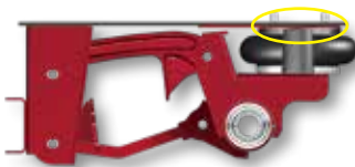
Figure A: Primary (airbag) bump stop engages
