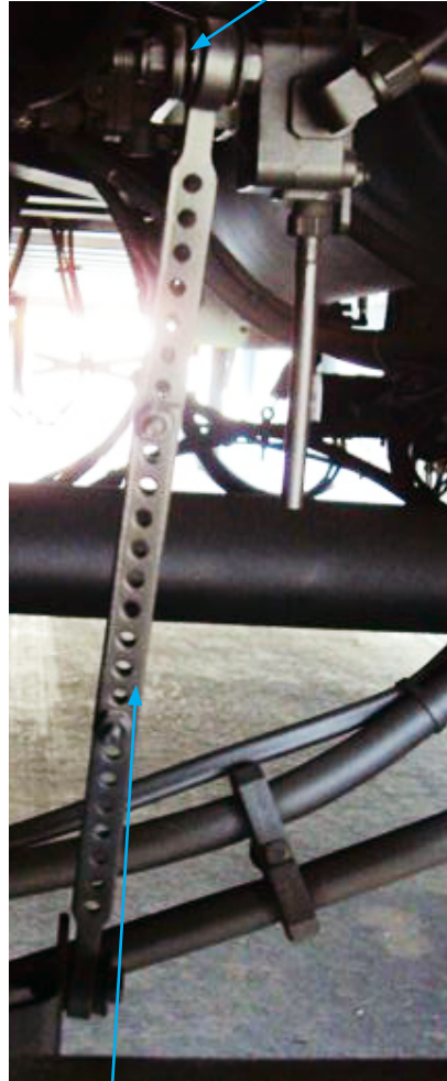
Linkage positioned non-vertical. Do not add lean or twist to linkage.
