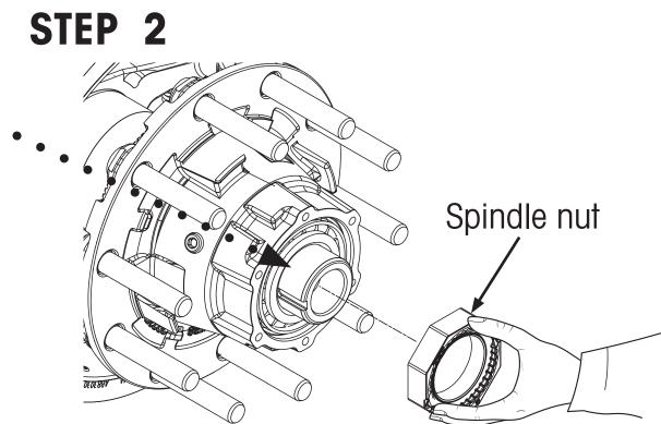
Torque to 200 ft. lbs. (271 Nm) while rotating hub 3 full turns
