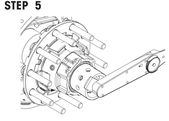
Torque to 50 ft. lbs. (68 Nm), then rotate hub 3 full turns. Repeat torque and rotations three more times. See note 1.
