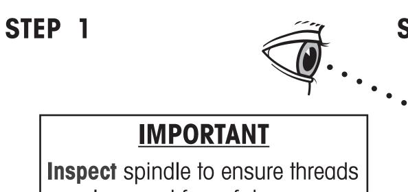
Inspect spindle to ensure threads are clean and free of damage and distortion. Ensure bearings are lubricated prior to installation.
