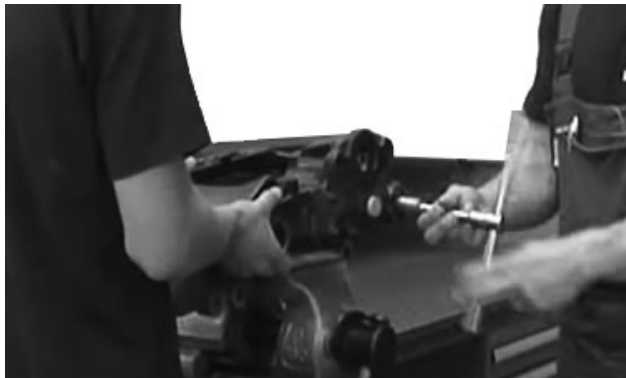
Figure 50: Supporting caliper while removing screws
