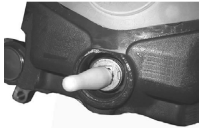
B. Placing mounting cap over adjuster
