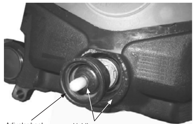
Figure 83: Installing adjuster boot
