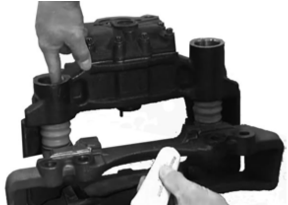
Figure 68: Greasing bore of guide pin cap
