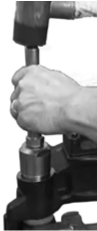
Figure 70: Using tool to install guide pin cap
