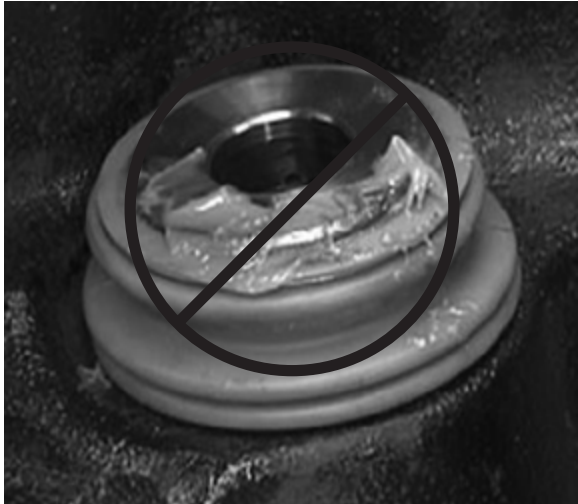
Figure 63: Excessive grease on guide pin and boot
