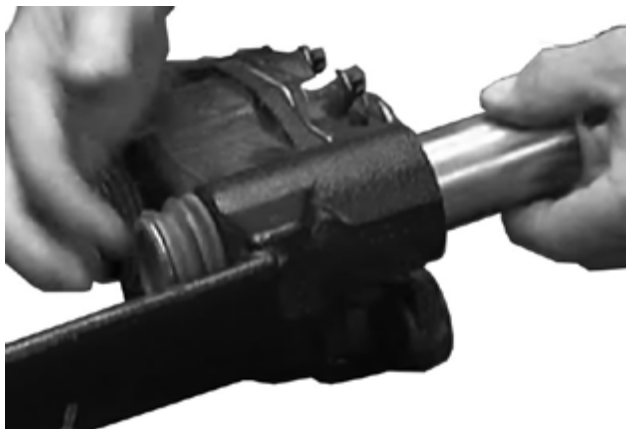
Figure 59: Inserting guide pin
