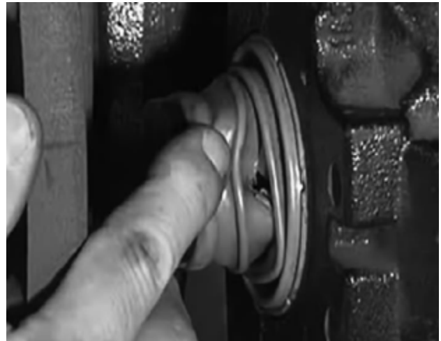
Figure 27: Adjuster piston boot damage
