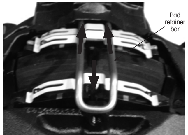
Figure 35: Installing pad retainer bar
