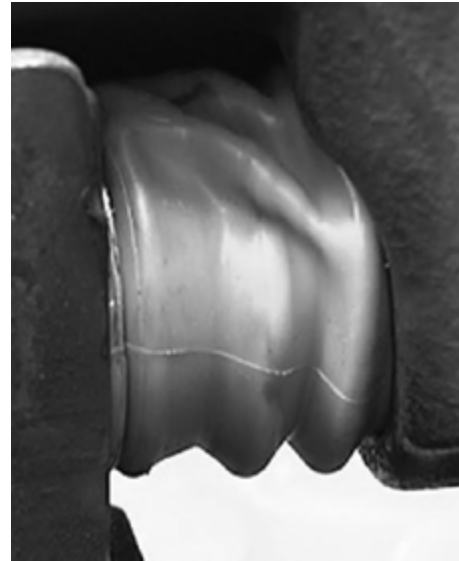
Figure 26: Twisted guide pin boot
