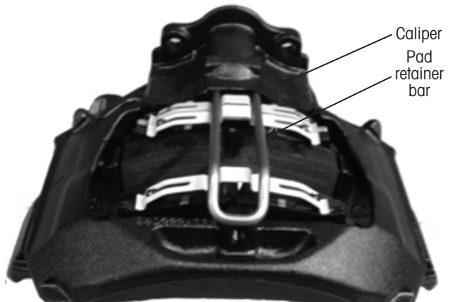
Figure 17: Loose pad retainer bar, prior to removal
