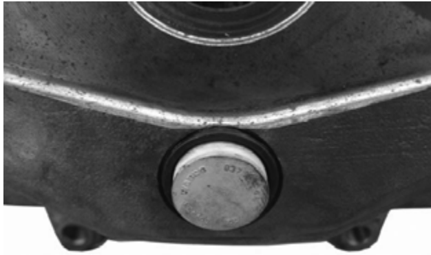
Figure 88: Adjuster plug properly inserted
