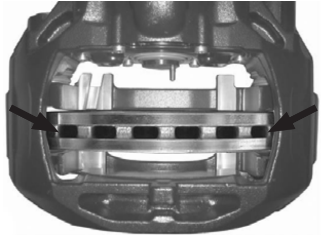
Figure 40: Positioning caliper over brake rotor
