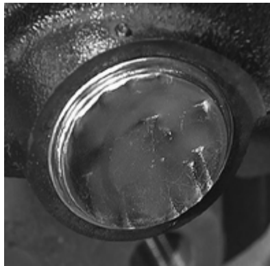
Figure 4: Damaged guide pin cap
