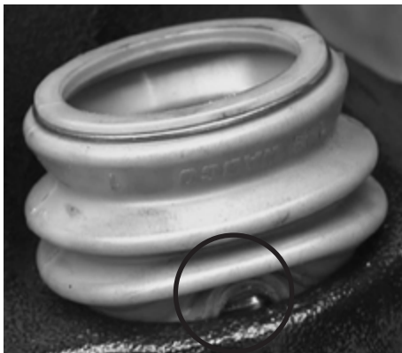
Figure 25: Improperly seated guide pin boot
