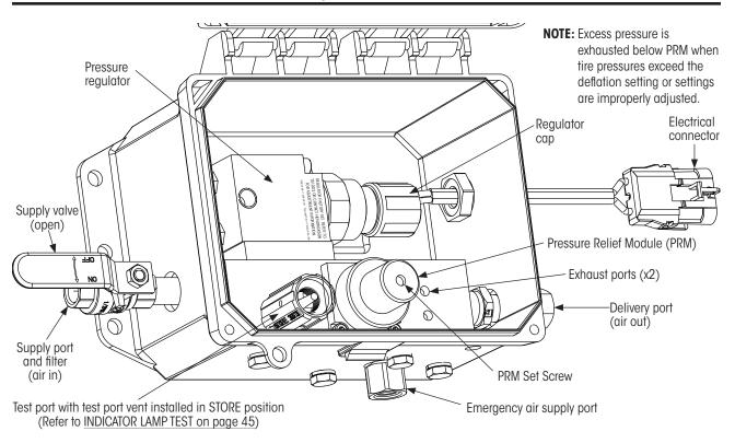
Figure 54: Setting TIREMAAX® PRO Inflation Pressure and Deflation Pressure
