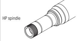
Figure 6: Axle spindle identification
