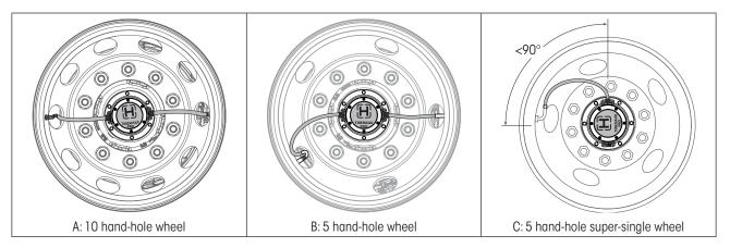
Figure 24: Properly clocking hubcap and wheels to prevent tire hose damage during operation
