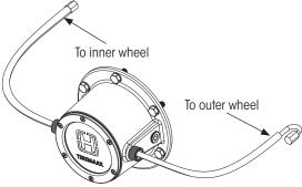
Figure 26: Dual tire hose to hubcap connection(s)
