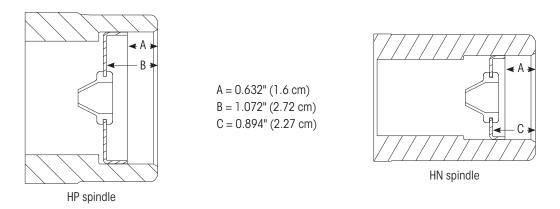
Figure 20: Recommended spindle plug depth (if not using plug tool shown in Figure 19)
