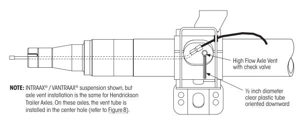
Figure 16: Typical axle vent installation
