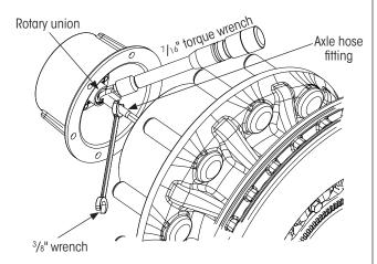
Figure 21: Hubcap to axle hose connection
