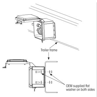
Figure 30: Controller mounted to trailer frame
