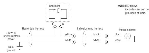
Figure 42: Typical wiring schematic for indicator lamp
