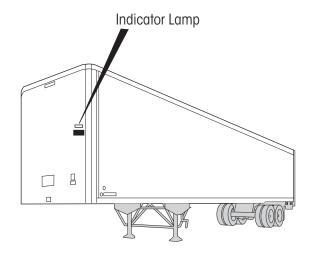
Figure 3: Indicator lamp typical location
