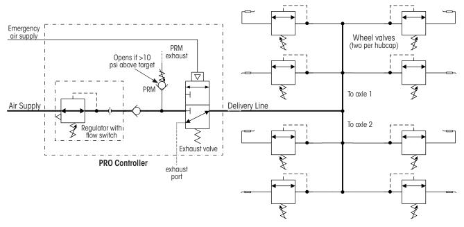
Figure 5: TIREMAAX PRO functional diagram
