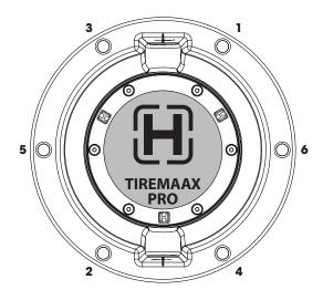
Figure 22: 6-bolt hubcap torque pattern
