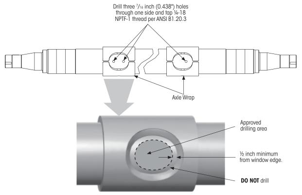
Figure 7: INTRAAX®/VANTRAAX® suspension axle drilling details
