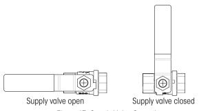
Figure 47: Supply Valve Operation
