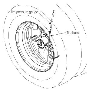
Figure 50: Manually checking tire pressure
