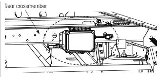
**NOTE:** Four holes are provided for mounting controller to rear crossmember.
