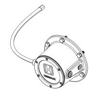
Figure 27: Super-single tire hose to hubcap connection
