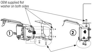
**NOTE:** TIREMAAX® PRO only. Use existing fasteners at bottom of controller. Remove, then replace after positioning on bracket. Torque to 60±12 in. lb. (8±2 Nm).
