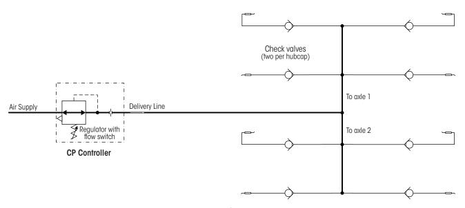
Figure 4: TIREMAAX CP functional diagram
