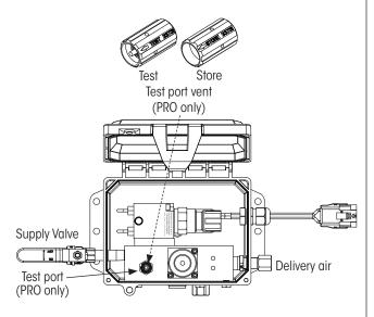
Figure 48: TIREMAAX® PRO controller with test port vent
