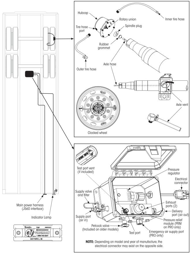
Figure 1: TIREMAAX® components (PRO controller shown)
