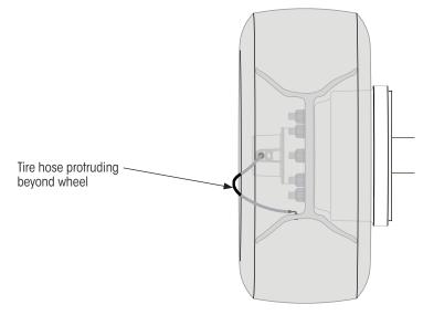
Figure 23: Improper tire hose installation (super single shown)
