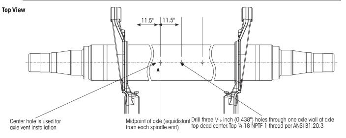
Figure 8: Hendrickson TRLAXLE® drilling details
