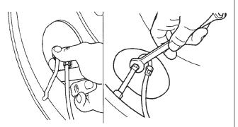
Figure 25: Attaching tire hoses to tire valve stem
