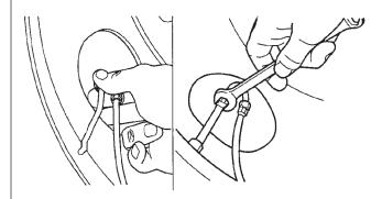
Figure 57: Reattaching tire hoses to tire valve stem
