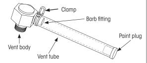
Figure 17: INTRAAX®/VANTRAAX®/ULTRAA-K® axle vent assembly
