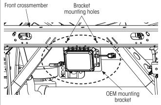
**NOTE:** Holes are also provided for mounting an optional OEM bracket to the front crossmember.
