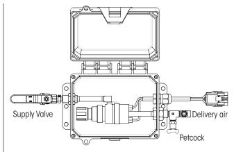
Figure 49: TIREMAAX controller with petcock (CP shown)
