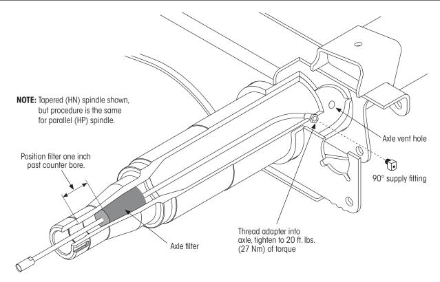
Figure 10: Installed position of axle hose assembly
