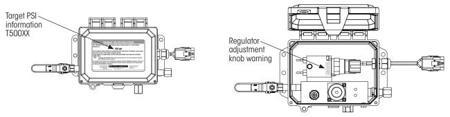
Figure 46: Controller decal locations (Installed by Hendrickson)
