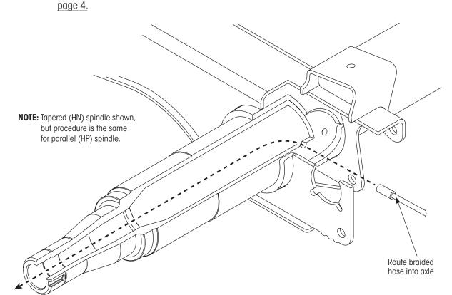
Figure 9: Routing axle hose
