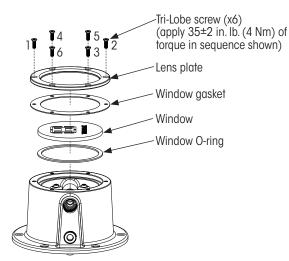
Figure 56: Hubcap window assembly
