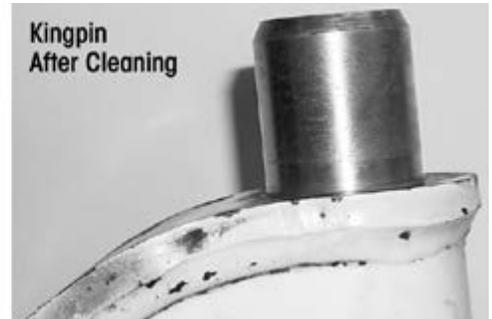
2. Inspect the kingpin for wear or damage. Use a micrometer and measure the upper and lower kingpin in two locations. Positions must be 90° opposed from each other. If the kingpin has less than 1.802" diameter, replacement of the axle is necessary, see Figures 9-46 through 9-49.
