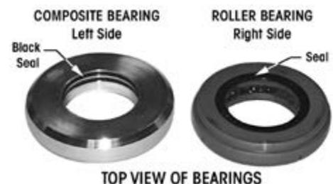
bearing is installed on the right side of the axle, see Figure 9-67. DO NOT substitute aftermarket components when servicing.
