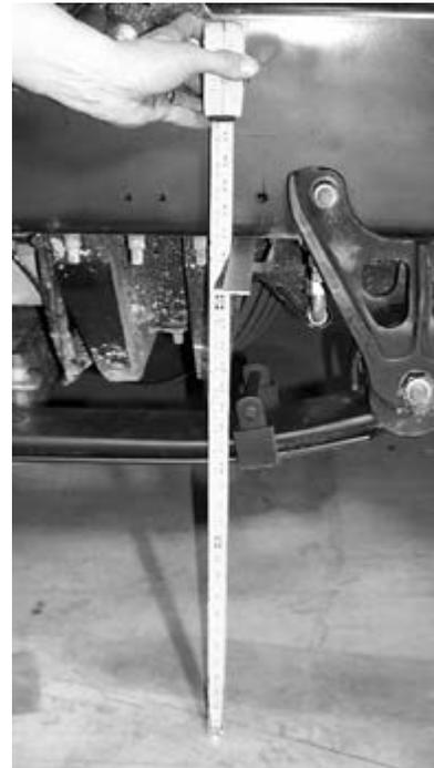
6. Affix a straight edge to the bottom of the frame rail behind the frame hanger, see Figure 8-18.
