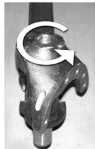
8. Check for the proper fit by rotating the knuckle assembly back and forth to verify there is no binding on the kingpin, see Figures 9-62 and 9-63.
