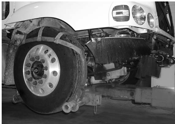
FIGURE 6-1 WHEEL LIFT METHOD
