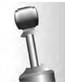
Damaged dust cover and / or shock body
