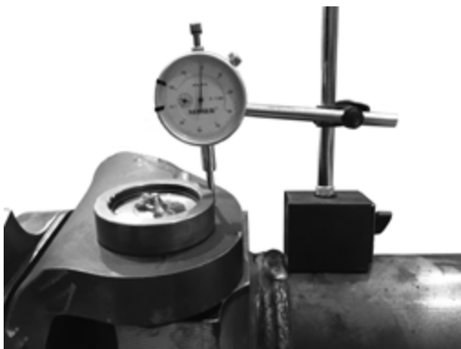
Figure 18: Checking steering knuckle vertical end play
