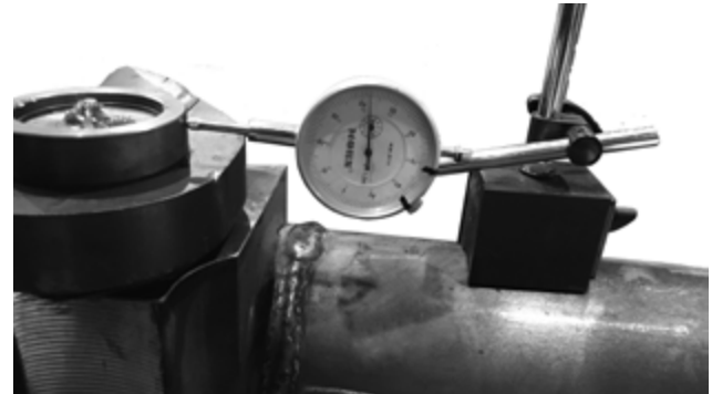
Figure 17: Checking upper kingpin bushing
