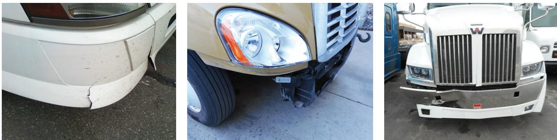
These photos show how whether a plastic or stainless steel bumper, damage is likely to occur on more than one component. With the consequential damage on multi-piece bumpers, it can actually be more cost effective to replace a one-piece bumper, in part, due to reduced assembly time.
