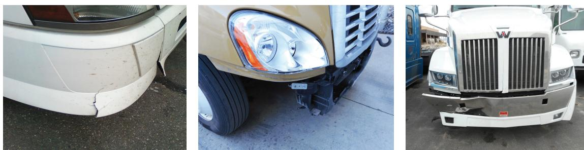
These photos show how whether a plastic or stainless steel bumper, damage is likely to occur on more than one component. With the consequential damage on multi-piece bumpers, it can actually be more cost effective to replace a one-piece bumper, in part, due to reduced assembly time.
