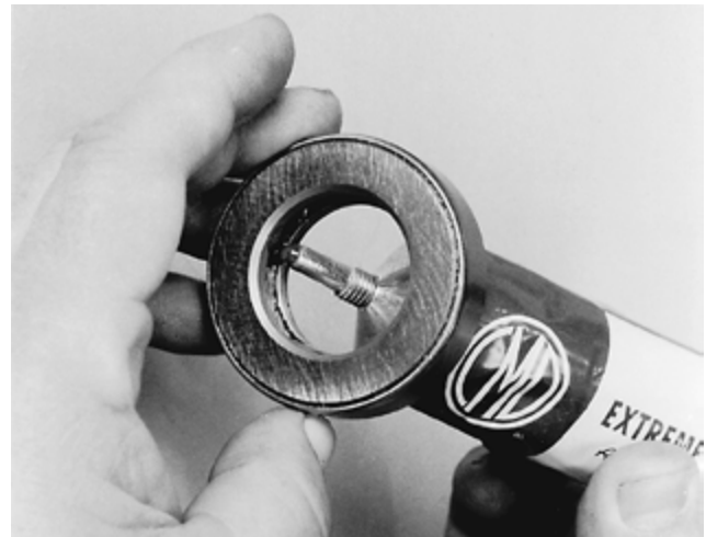
Figure 31: Applying lube to thrust bearing
