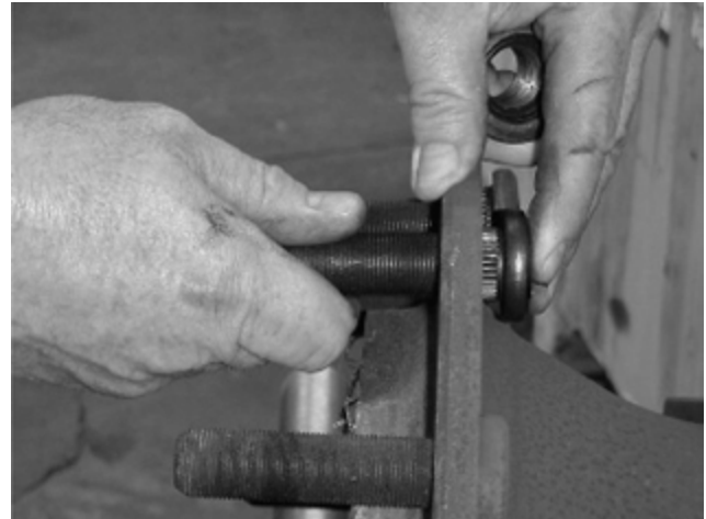
Figure 5: Installing new studs
