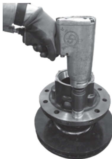
Figure 16: Stud draw-in process
