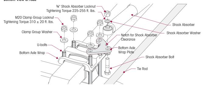
4. Ensure that the clamp group is properly aligned and the U-bolts are seated properly in the top pad, and the bottom axle wrap is centered on the top axle wrap, see Figure 4 and 5.
