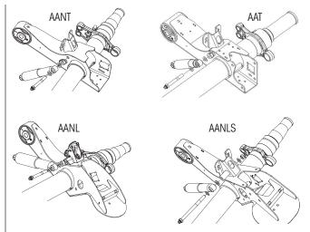
Figure 5: Sample lower shock mount hardware
