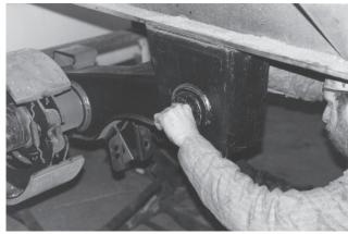
Figure 9: Installing new pivot connection hardware
