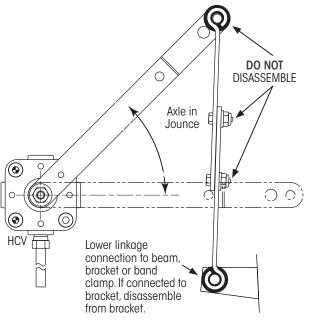
Figure 1: HCV linkage lower connection
