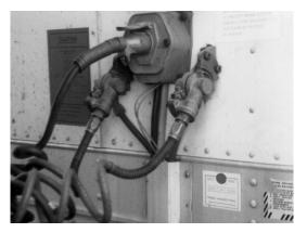
Figure 11: Trailer connections
