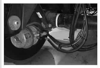
Figure 3: Brake chamber
