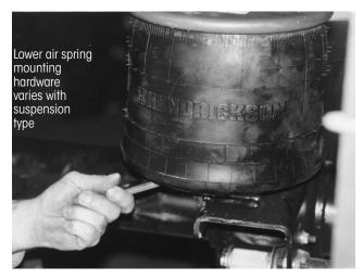
Figure 4: Air spring bottom fastener(s)
