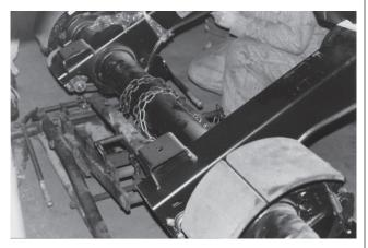
Figure 7: New HALFTRAAX<sup>™</sup> secured to transmission jack
