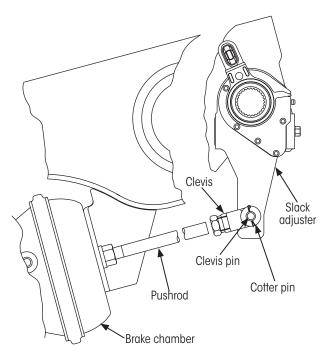
Figure 10: Brake chamber/slack adjuster connection
