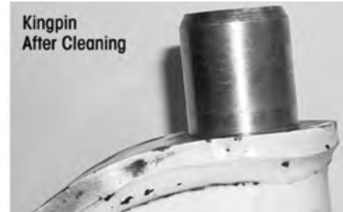
2. Inspect the kingpin for wear or damage. Use a micrometer and measure the upper and lower kingpin in two locations. Positions must be 90° opposed from each other. If the kingpin has less than 1.802" diameter, replacement of the axle is necessary, see Figures 9-54 through 9-57. **Kingpin minimum dimension is 1.802".**
