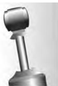
Damaged dust cover and / or shock body
