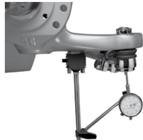
11. If there is any movement in the tie rod assembly, install a magnetic based dial indicator on the Ackermann arm, see Figure 7-10.
