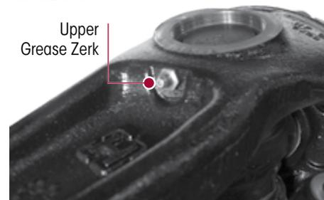
2. Prior to greasing the kingpins on the vehicle, the suspension must be in a loaded condition.
