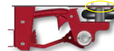
Figure A: Primary (airbag) bump stop engages
