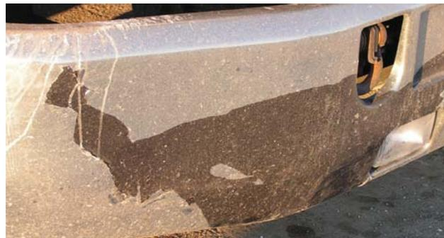
**Flange and Mounting Hole Cracking**
