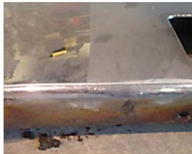
Corrosion on bottom flange of the bumper
