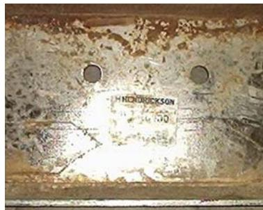
Corrosion on back side of the bumper
