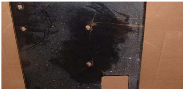
Flange cracking due to damage originating at other locations on the bumper
