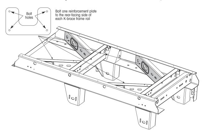
Effective immediately, Hendrickson will begin sending reinforcement kit S-27316-2 to all identified HKA250 suspension owners. Upon arrival, you are authorized to install or have these reinforcement plates installed.
