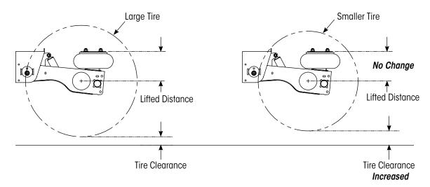
Reducing the tire size will also increase the suspension ride height when the axle is lowered. Exceeding the maximum allowed ride height could result in a loss of suspension capacity and damage to the suspension components. The maximum allowable suspension ride height should never be exceeded. Refer to L388 Recommended Ride Height Settings to determine the maximum ride height.
