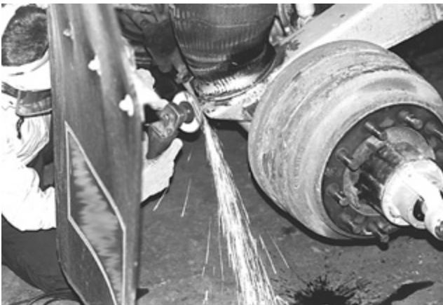
Figure 68: Preparing rear suspension beam ends
