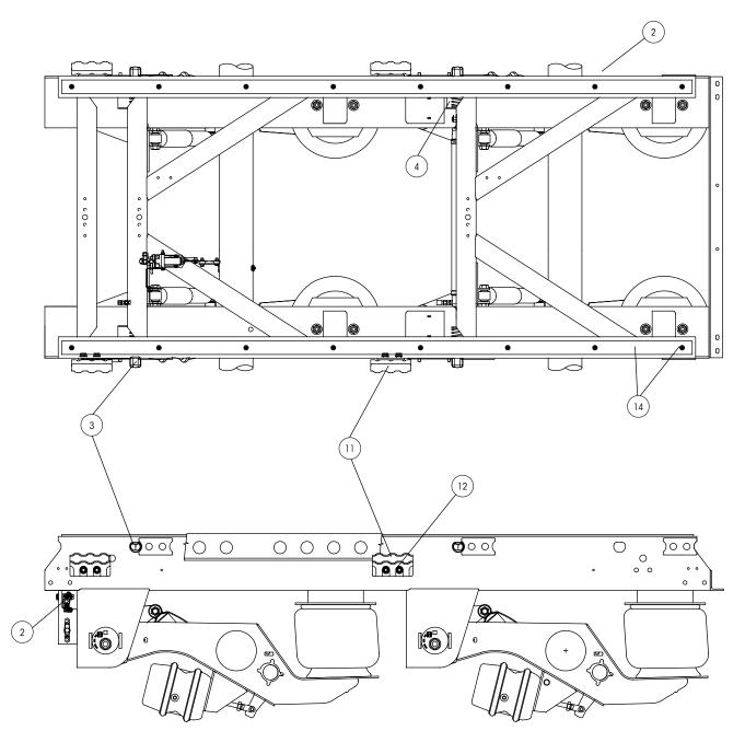
Note: Identification tag can be found on the roadside slider box rail above the front frame bracket. There will also be a blank INTRAAX® tag on the inside of the curbside beam.
