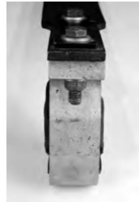
6. Tighten rear spring mount locknuts to  $95 \pm 15$  foot pounds torque.
