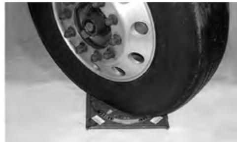
3. If the vehicle is equipped with power steering, check the pressure relief in the power steering system and reset if necessary. Refer to vehicle manufacturer regarding the subject: Adjusting the Pressure Relief in the Power Steering System.
