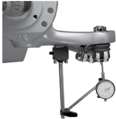
11. If there is any movement in the tie rod assembly, install a magnetic based dial indicator on the Ackermann arm, see Figure 7-9.
