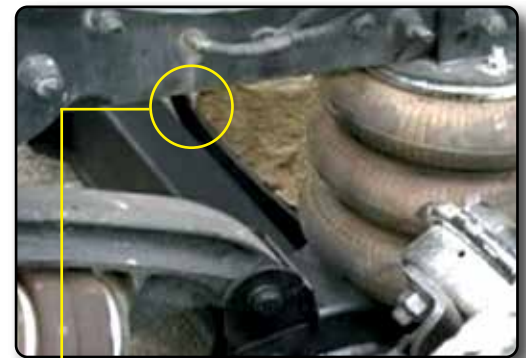
CTR absorbs strike and returns to original state.
