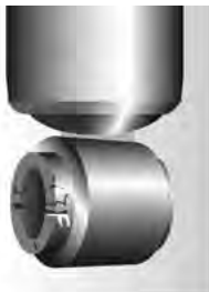
Damaged upper or lower bushing
