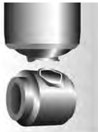
Damaged upper or lower mount
