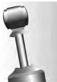
Damaged dust cover and / or shock body
