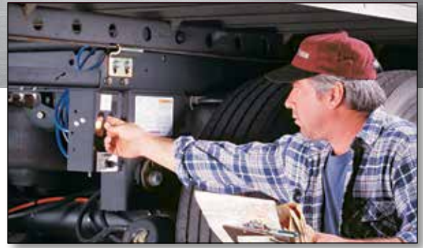
QUIK-DRAW allows drivers to disengage the slider's lock pins using only fingertip effort.
