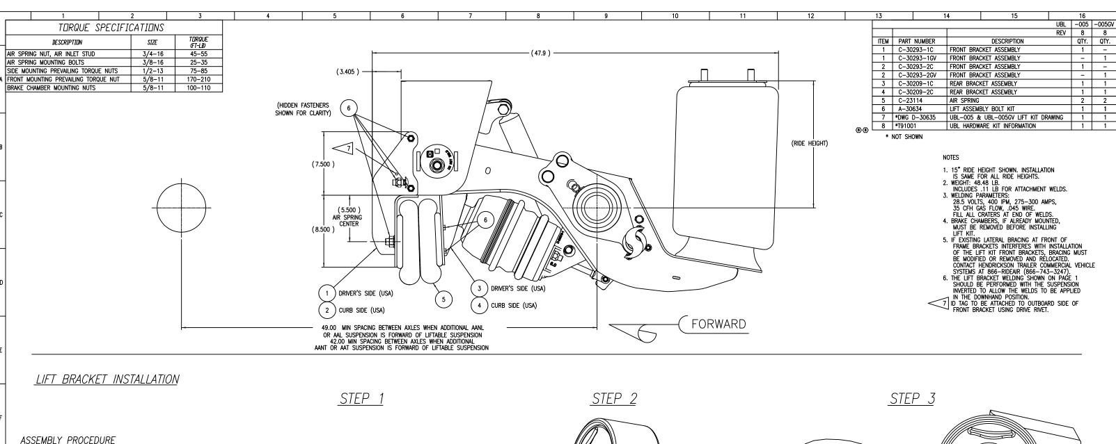
\*UBL CANNOT BE INSTALLED WITH SUSPENSION ASSEMBLED TO FRAME BRACKET (UNITIZED), AS EXCESSIVE WELDING HEAT WILL DAMAGE THE PIVOT BUSHING. SUSPENSION MUST BE DISASSEMBLED FROM FRAME BRACKETS BEFORE WELDING.
