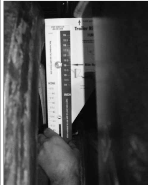
Figure 3: Using gauge to measure ride height
