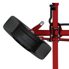
Optimized steering system — 55-degree wheel cut
