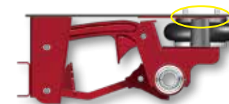
Figure A: Primary (airbag) bump stop engages
