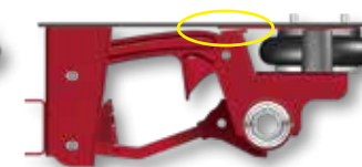
Figure B: Under extreme load, secondary bump stop engages
